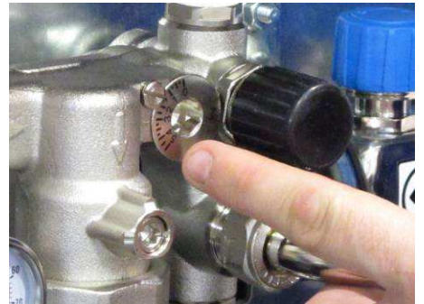
Do not adjust the primary water temperature regulator. The factory setting is 3. The unit is delivered with the black bypass knob closed. Once system is filled open by 1/16 of a turn anti clockwise. This allows water through the blending valve in the event that all circuits are closed.
