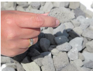
Foam glass aggregate size typically between 10-60mm
